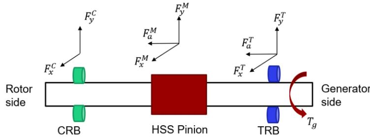
Figure 14: Freebody diagram of HSS.
