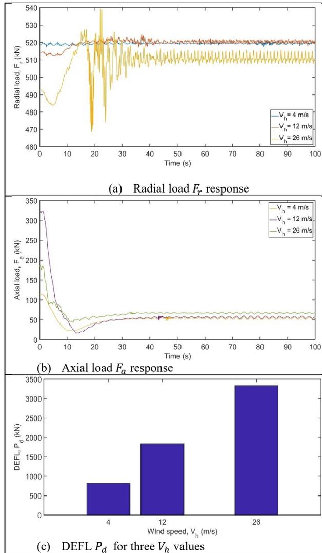
Figure 11: DLC 3.1 load case, maximum main bearing loads.
