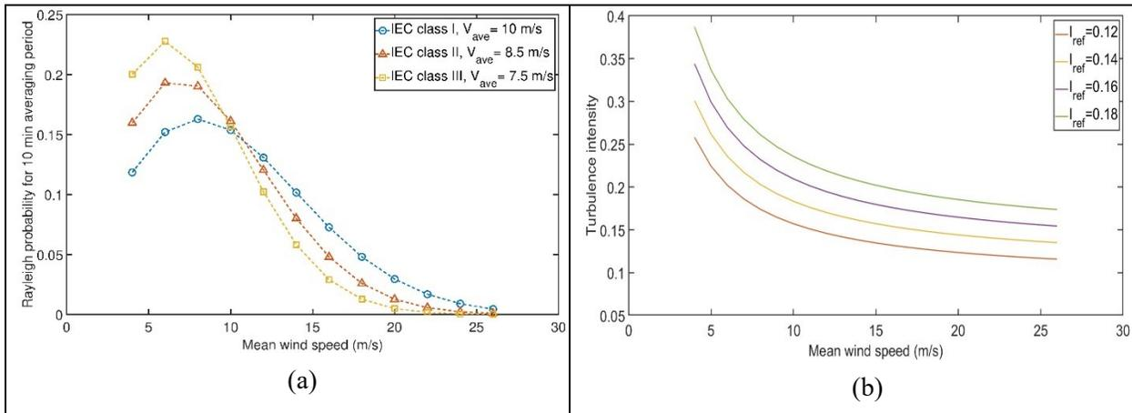
Figure 1: (a) Frequency of occurrence of 10-min mean wind speed  $V_h$  for different IEC wind classes and (b) Turbulence intensity ( $I$ ) as a function of  $V_h$ .
