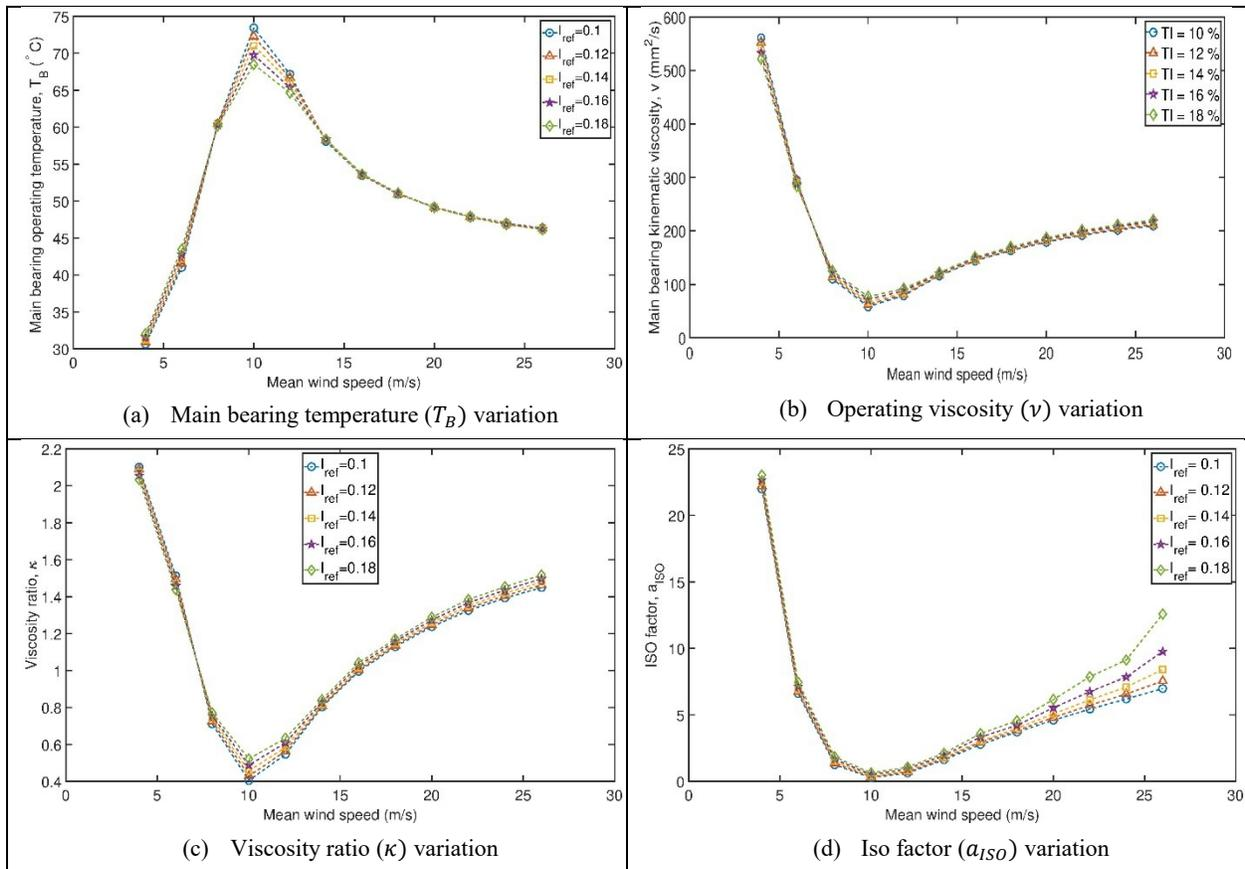
Figure 7: Variation of the main bearing operational parameters with mean wind speed ( $e_c = 0.7$  (normal cleanliness),  $T_A = 22^\circ$  C).
