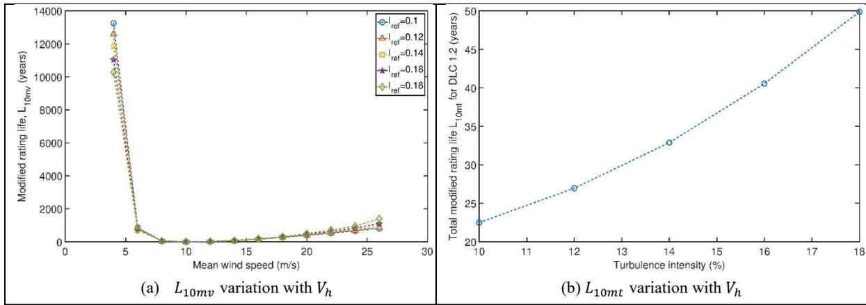
Figure 8: Influence of the turbulence intensity on the main bearing modified rating life for DLC 1.2 load case ( $e_c = 0.7$  (normal cleanliness),  $T_A = 22^\circ C$ ,  $V_{ave} = 8.5$  m/s).
