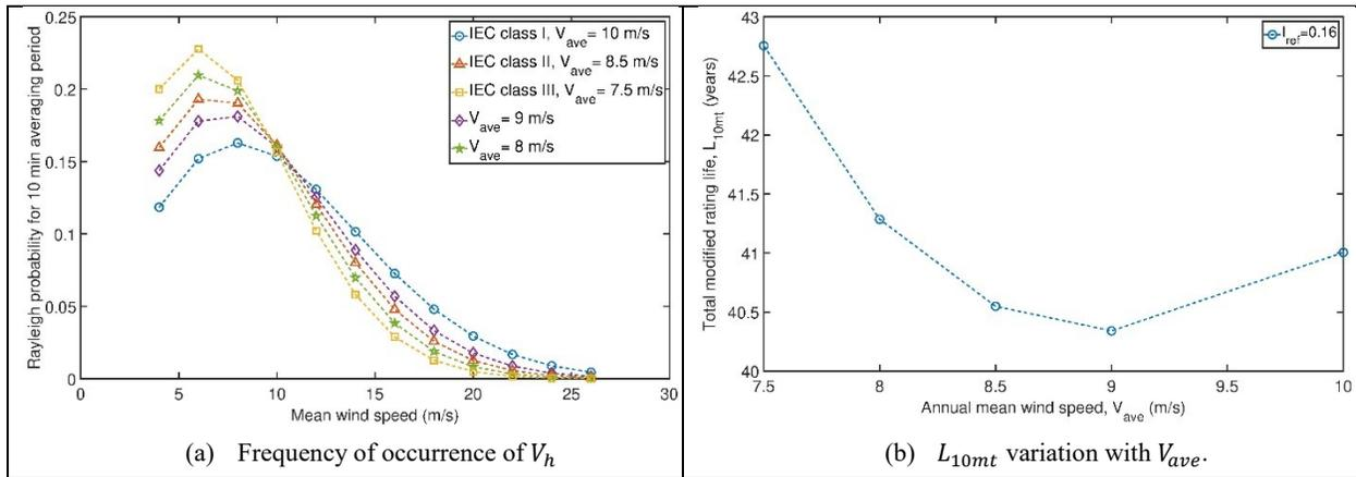
Figure 9: Influence of the different IEC wind classes on the main bearing modified rating life for DLC 1.2 load case ( $I_{ref} = 0.16, e_C = 0.7, T_A = 22^\circ C$ ).
