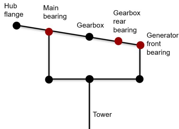
Figure 3: HAWC2 representation of the drivetrain of the SWT-2.3-93
