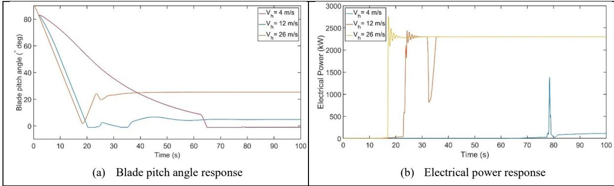
Figure 10: DLC 3.1 start-up load case
