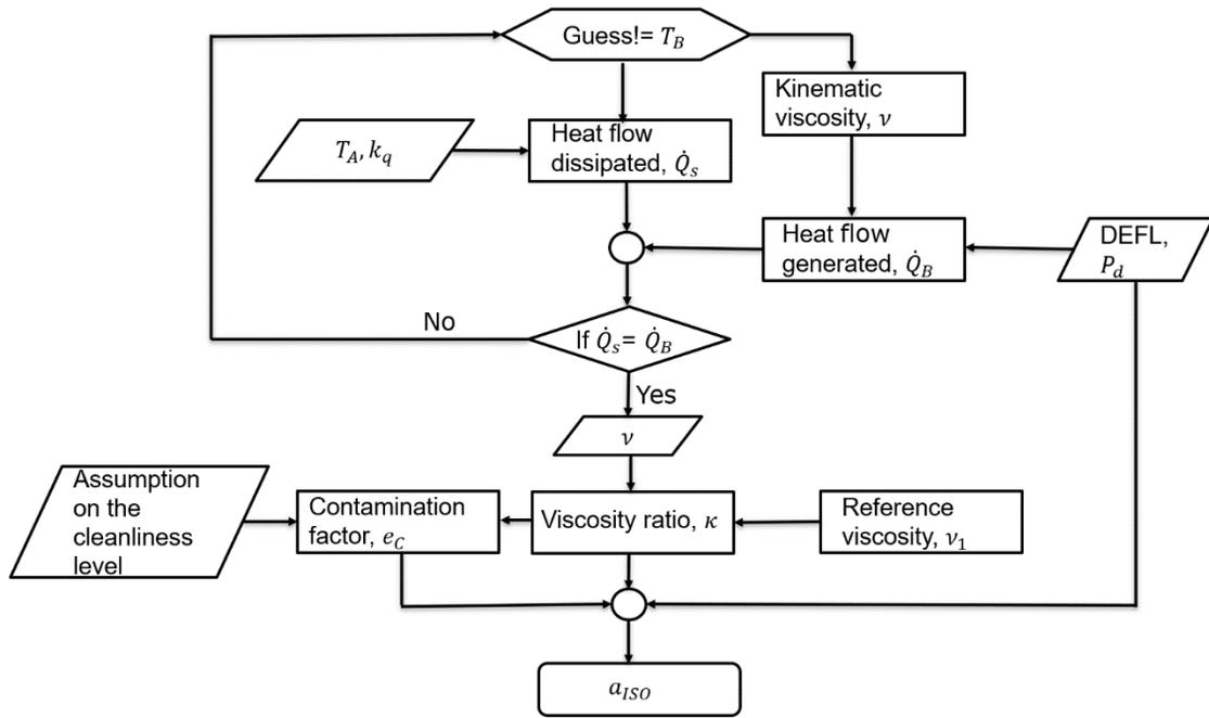
Figure 4: The life modification factor,  $a_{ISO}$  calculation algorithm
