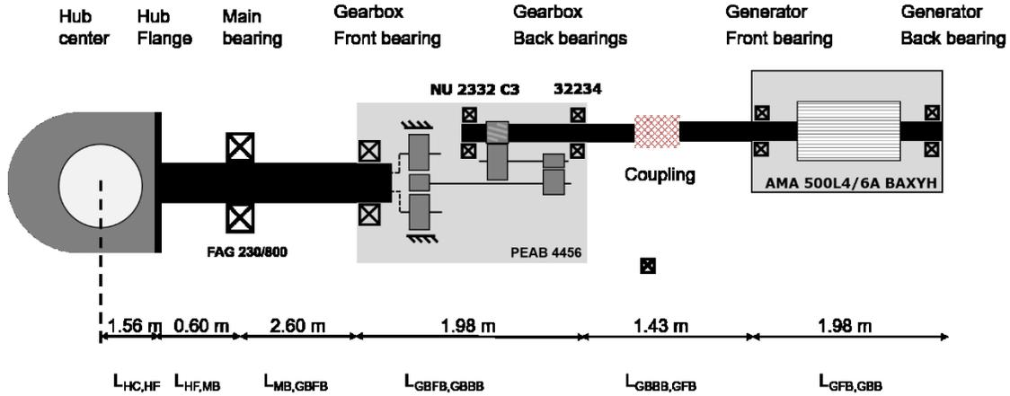
Figure 2 Proposed drivetrain layout of the Siemens SWT-2.3-93 turbine based on the spare part report of SparesInMotion (SparesInMotion, 2023)
