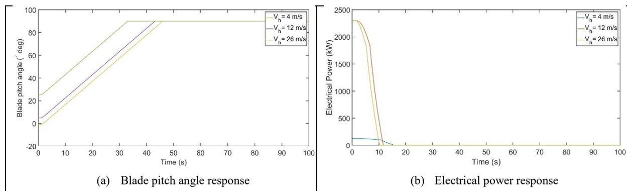
Figure 12: DLC 4.1 normal shutdown load case
