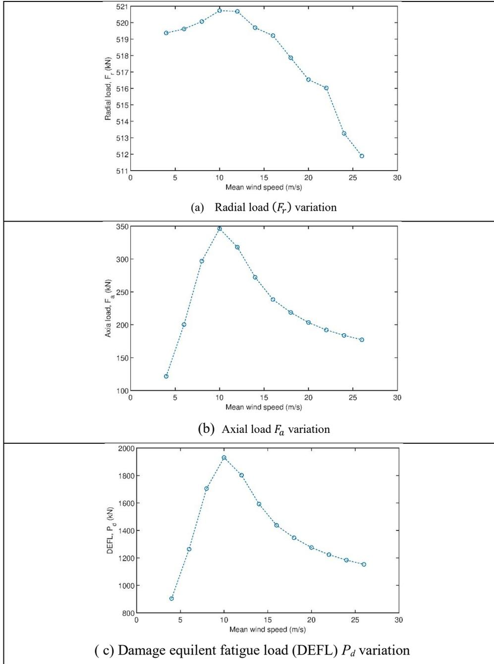
Figure 5: Main bearing loads as a function of mean wind speed for DLC 1.2 load case with  $V_{ave} = 8.5$  m/s, and  $I_{ref} = 0.16$ .
