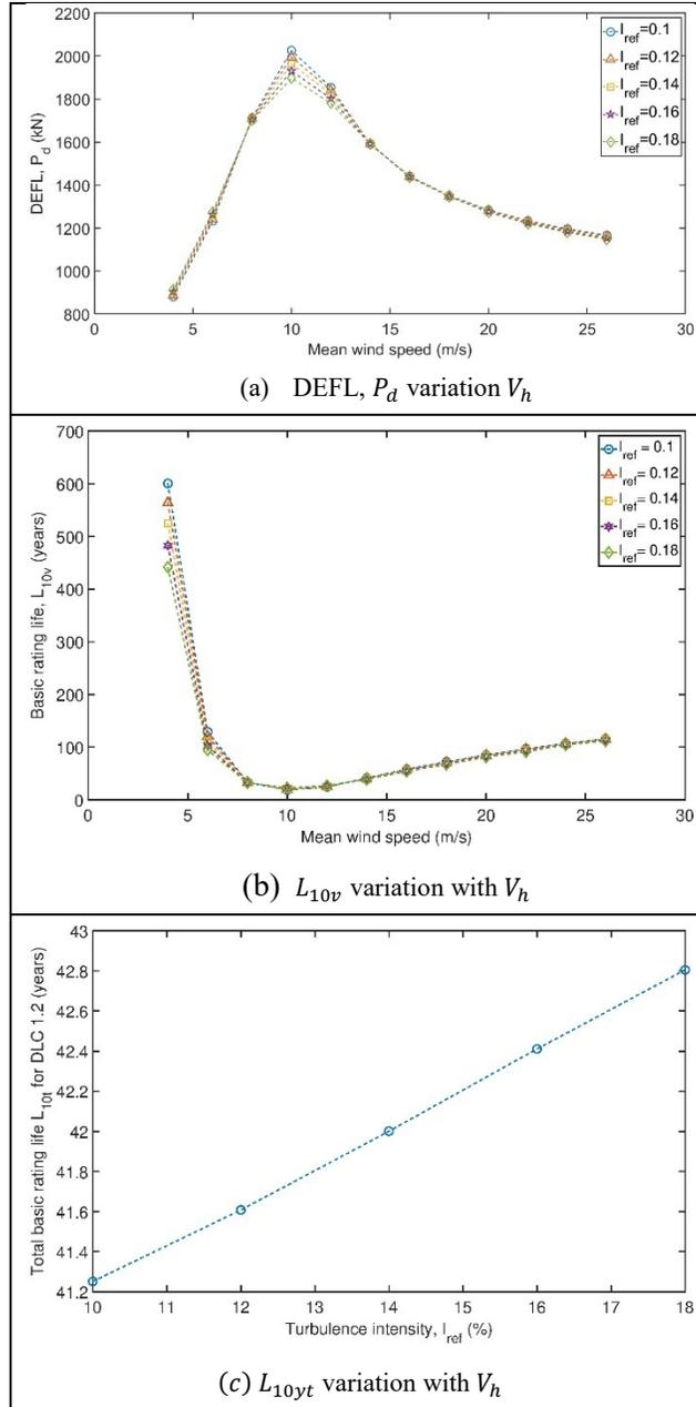
Figure 6: Influence of the turbulent intensity on the main bearing basic rating life for DLC 1.2 load case with  $V_{ave} = 8.5$  m/s.
