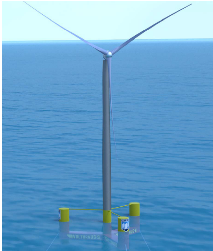
Figure 3.1: Umaine Semisubmersible with IEA 15 MW Turbine (Allen et al., 2020; Gaertner, 2020)
